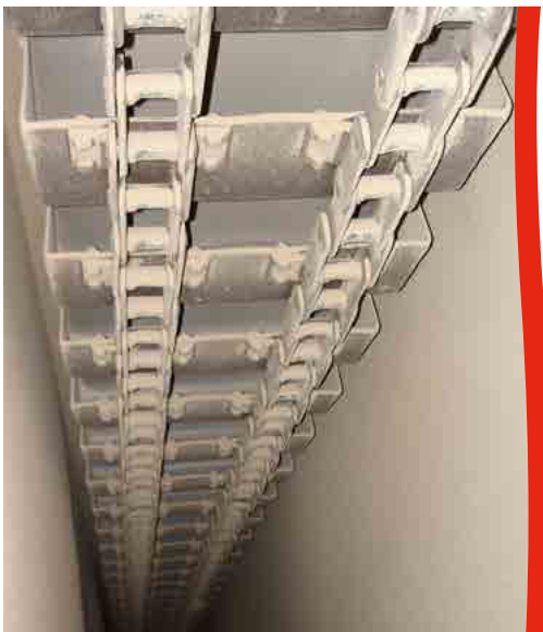
Chain for elevator
